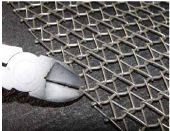
Figure 2.1 Cut Wire at Ball Joint
