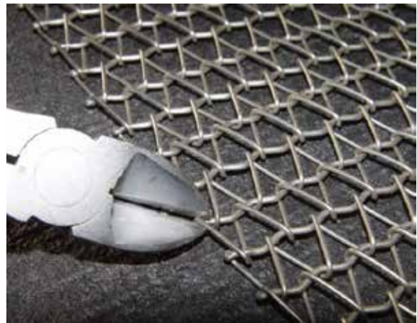
Figure 2.1 Cut Wire at Ball Joint
