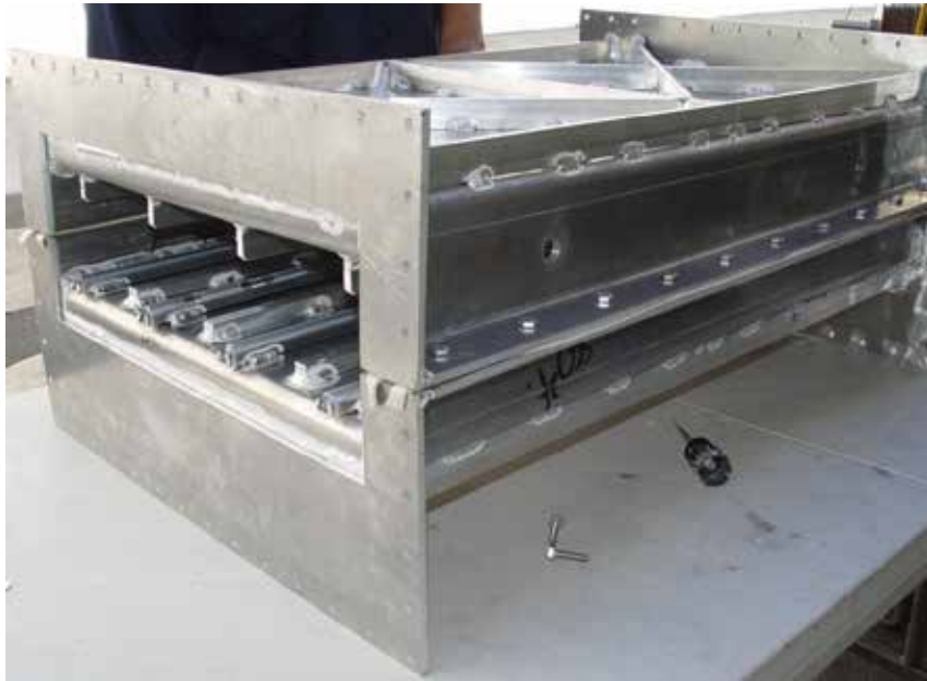
New Cooling Section with quartz rods
