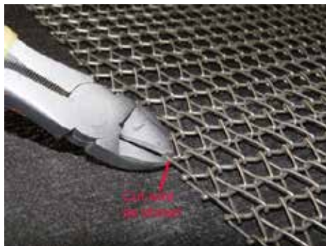
Making a Belt Splice Rod
