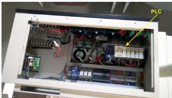
Figure 3-1 Remove control console top access panel
