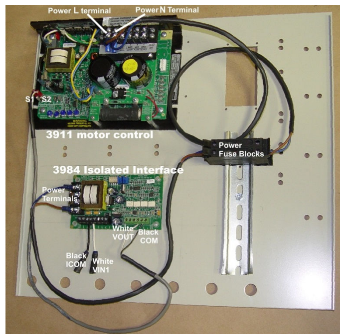
Figure 1 Motor control Panel Layout
