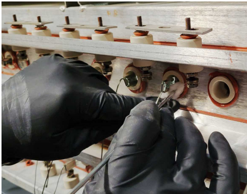
Figure 4-4: Insert seal around lamp
