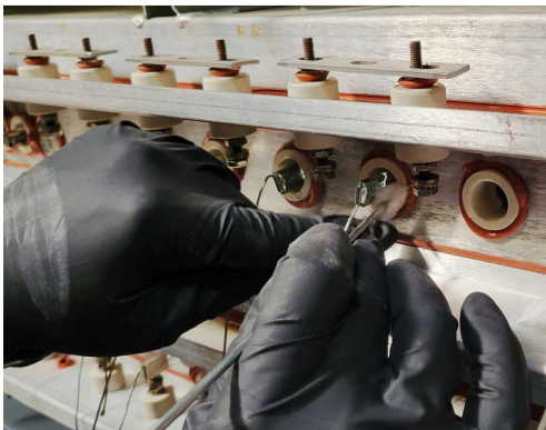
Figure 4-4: Insert seal around lamp
