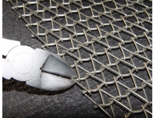
Figure 3-3 Cut Wire at Ball Joint
