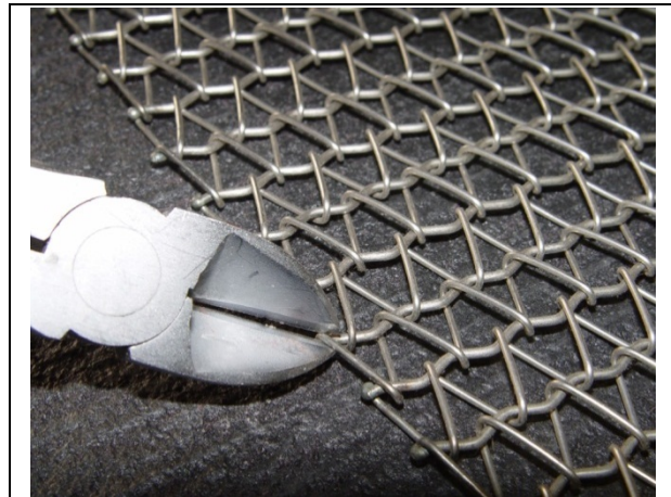
Figure 3-4 Cut Wire at Ball Joint
