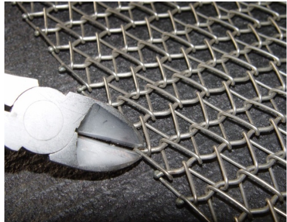
Figure 2.1 Cut Wire at Ball Joint
