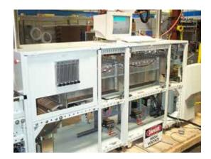
3.2 Unplug computer monitor and remove from furnace.
