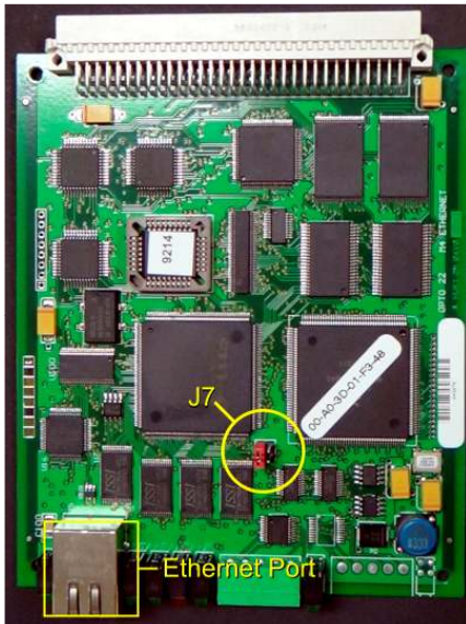
Figure 3-16 Location of J7 Jumper J7 in Normal RUN Position
