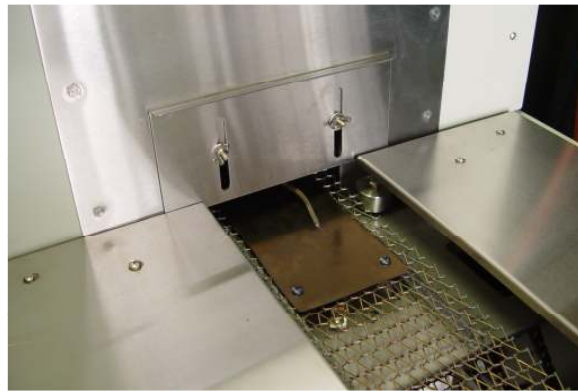
Figure 5-12 Sample plate exiting furnace
