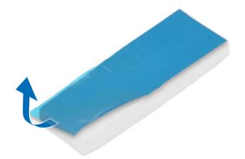
4. Place the rubber on the system board [1] and peel the adhesive tape (pink) from the rubber [2].
