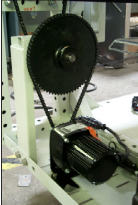
Figure 3-9: Conveyor Belt Motor
