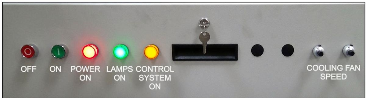
**Figure 2-2 Control Console Furnace Power ON and OFF & Indicator Lights**
