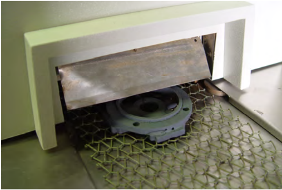
Figure 8-11 Brass forging sample exiting furnace
