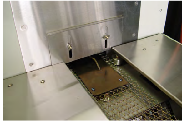
Figure 8-12 Sample plate exiting furnace
