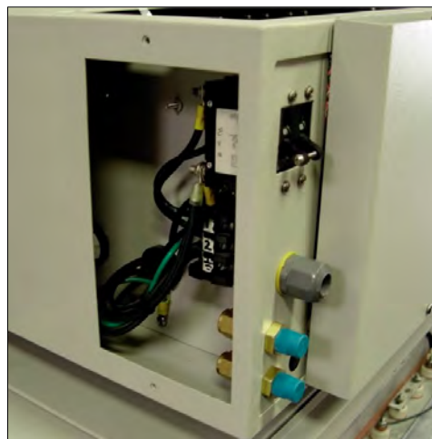
Figure 0-5 Control Enclosure showing 3 options: Circuit Breaker; Dual Process Gas; & Sample Port
