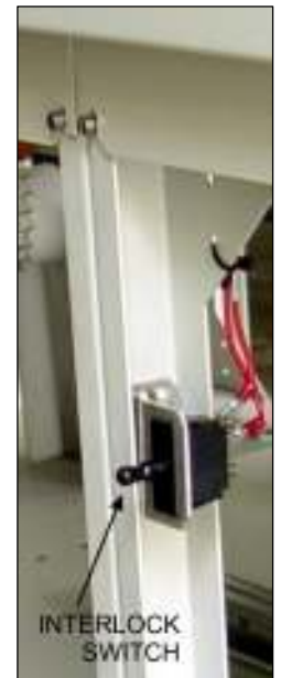
Figure 3-2 Lower Panel Interlock
