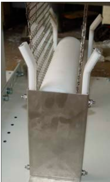
Figure 7-22 Belt Weight in Place
