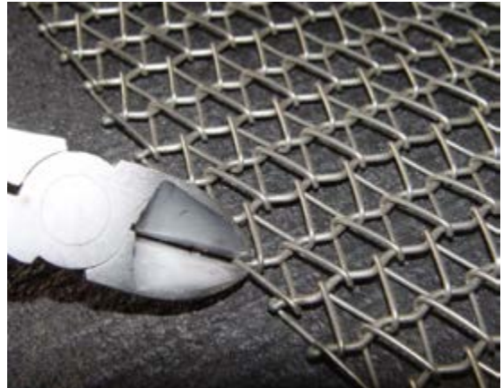
Figure 7-14 Cut Wire at Ball Joint
