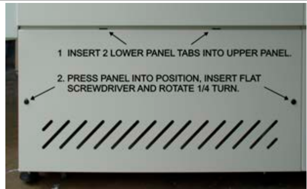
Figure 7-7 Lower Access Panel Installation
