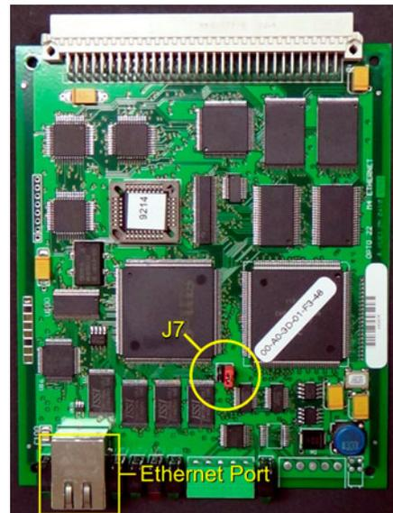
**Figure 3-30** J7 Jumper at Module RESET
