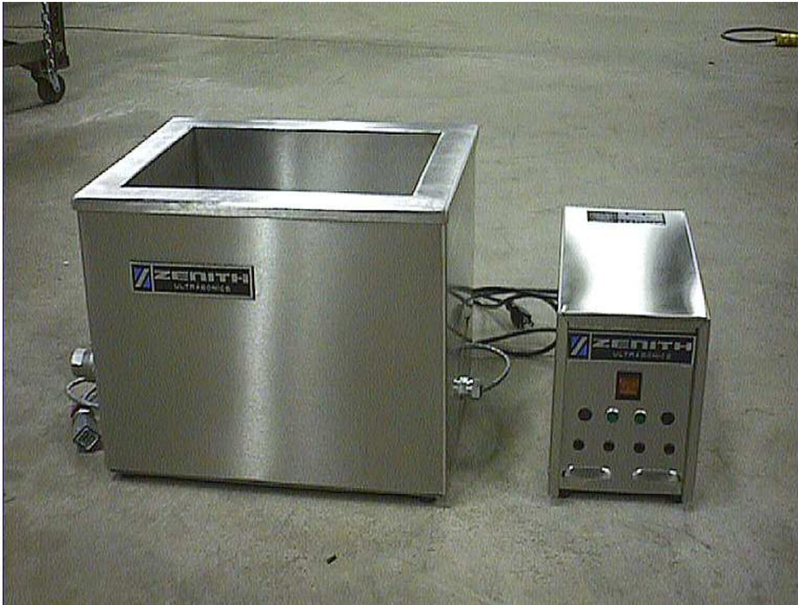
*Ultrasonic Cleaning Tank (left) and 80Khz OMEGA-HF Generator.*
