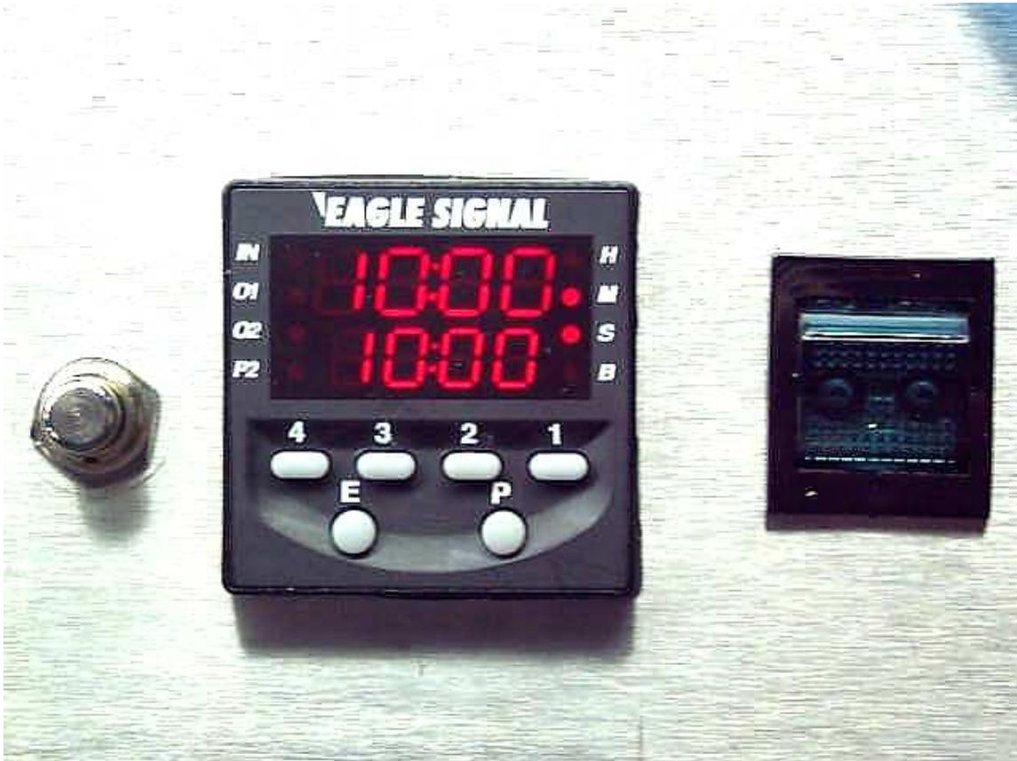
The digital timer is a black device that will be mounted to the control panel, and will have a digital backlit LED display. The large red on top of the smaller numerals in the center of the display represents the timer current value, while the smaller numerals at the bottom of the display represents the current set-point of the timer.
