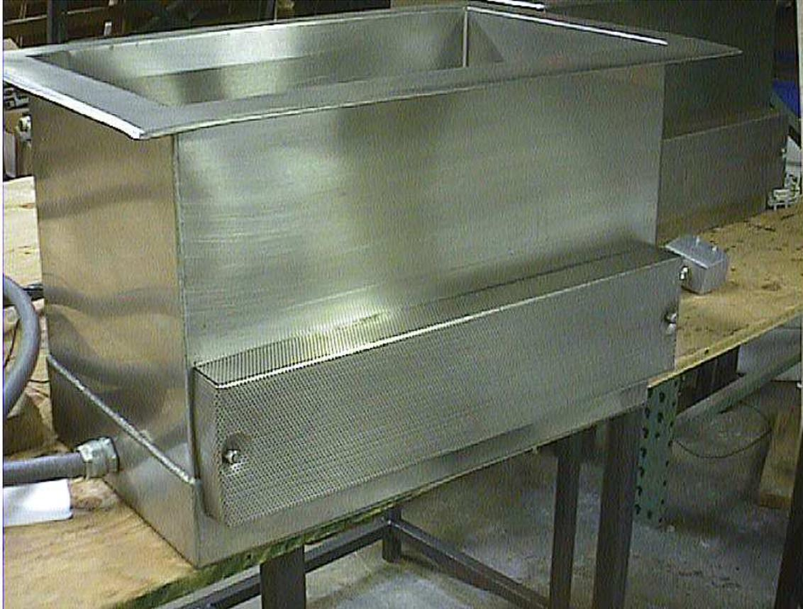
**Bar Heater Unit Mounted to Outside of Tank Keeps Tank Interior Smooth.**
