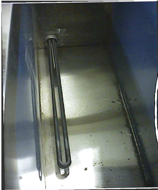
**Immersion Heater Bars Extend Into Tank to Heat Fluids**
