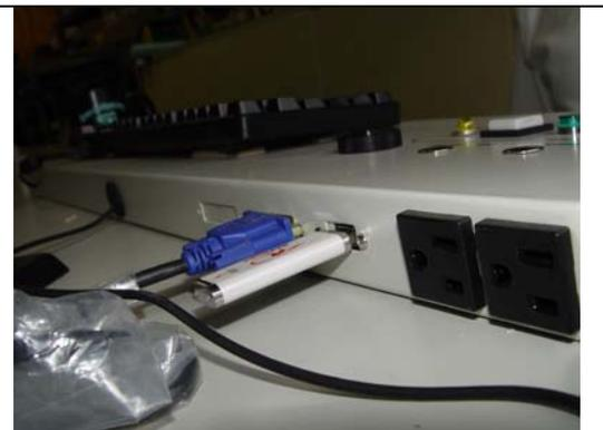
Figure 2.1.2 Control Panel, Rear showing monitor and USB ports.
