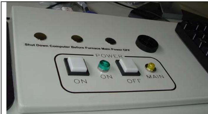
Figure 2.1.1 Control Panel showing Main Power ON and OFF and Indicator Lights
