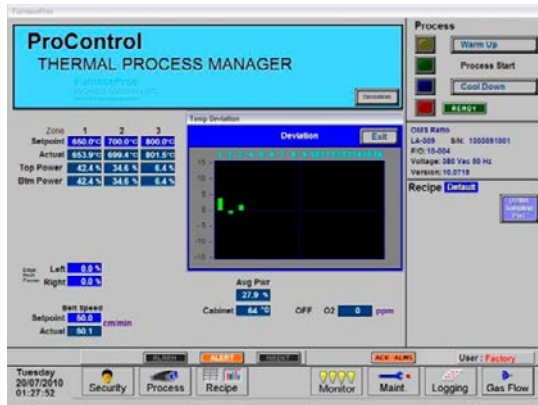
LA-306 Software Process Screen During @ 800 C Profile, Belt Speed: 50 cm/min
