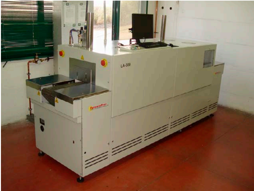
LA-309 Nitrogen High Temperature Furnace at Customer Site (3250 mm L x 960 mm W x 1700 mm H)
