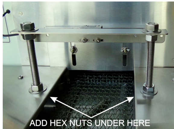
Figure 2-24 Install SENSLAS bracket
