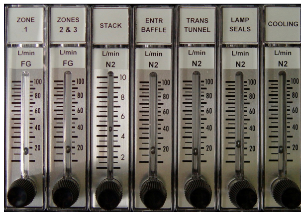
Figure 1-21 Gas Flowmeters - Dual Gas
