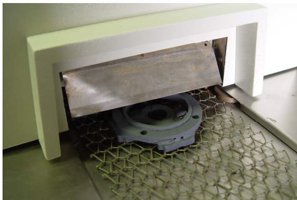
Figure 9-11 Brass forging sample exiting furnace
