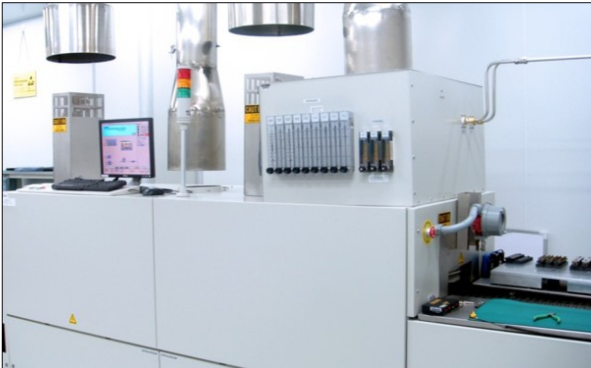
Figure 2-30 Typical Hydrogen Furnace Process Gas Exhaust Connection
