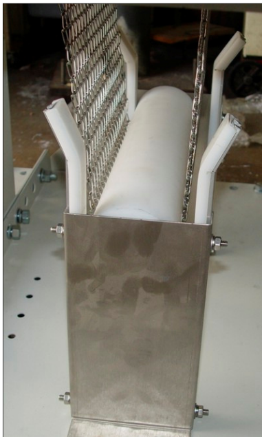
Figure 2-11 Belt Weight in Place
