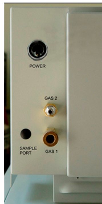
Figure 2-20 Process Gas Connections - Dual Gas
