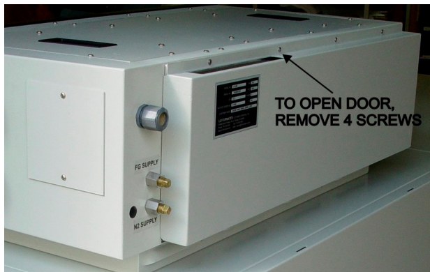
Figure 7-4 Control Enclosure Access Door Closed
