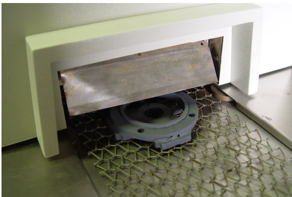
Figure 9-11 Brass forging sample exiting furnace
