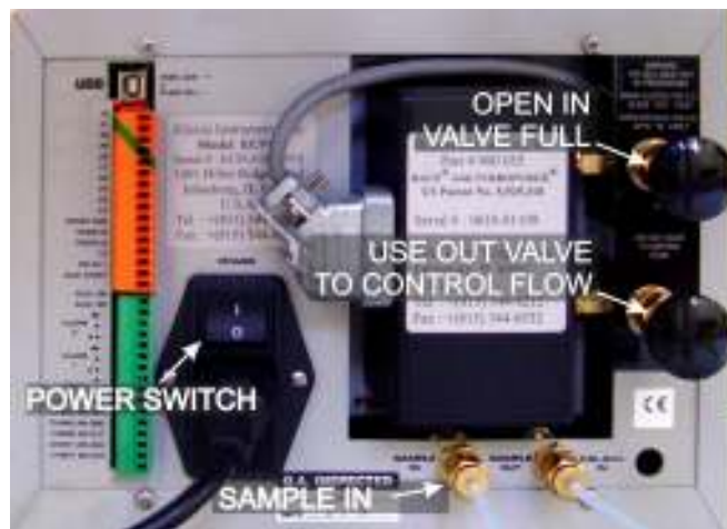
Figure 6-15 EC913 Oxygen Analyzer Rear Controls Pre-2016 Analyzers (Newer, see Figure 6-13)
