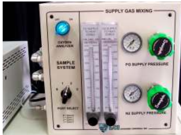
Figure 6-14 Sample System control panel (shown with Supply Gas Mixing System)
