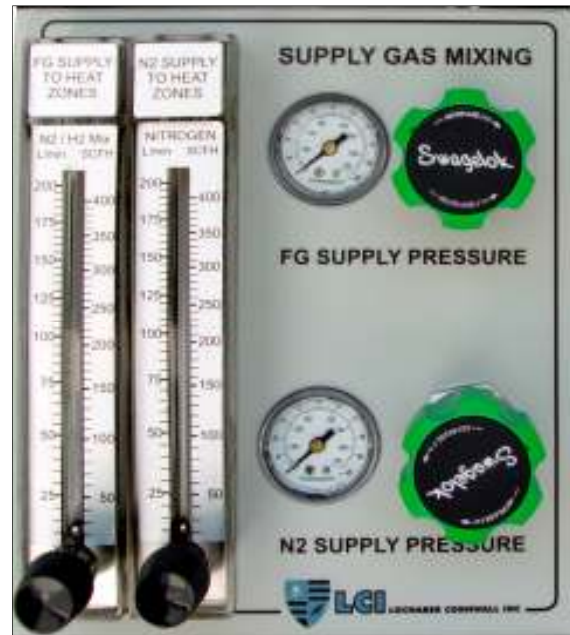
Figure 6-7 Supply Gas Mixing System Control Panel
