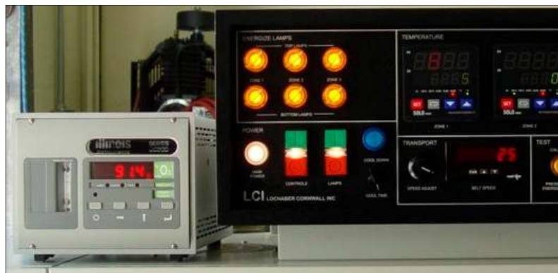
Figure 6-11 Oxygen Analyzer next to Control Console
