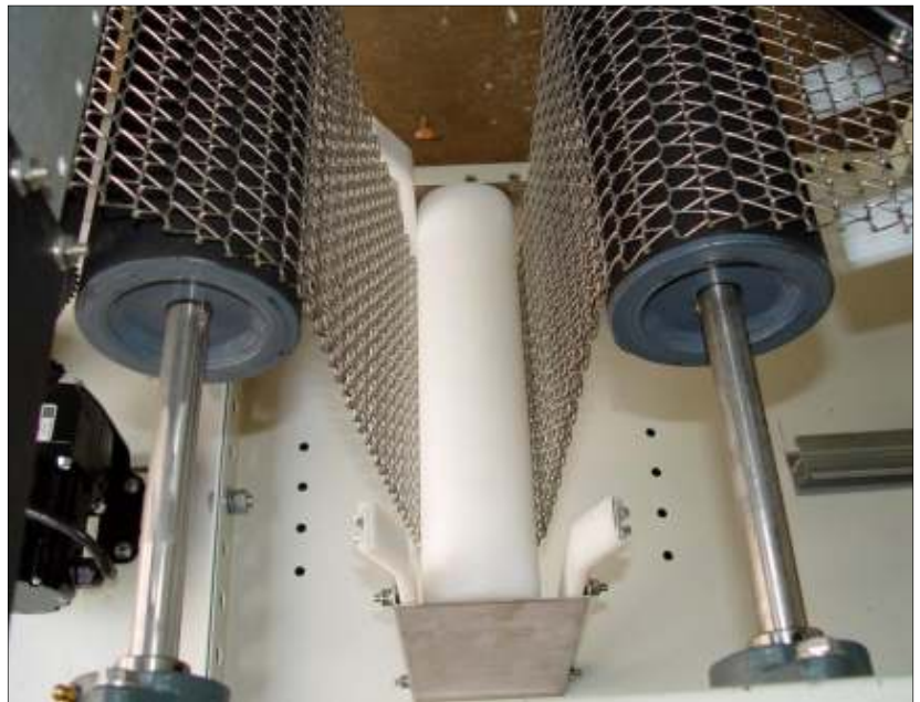
Figure 2-12 Proper Alignment of Belt Weight
