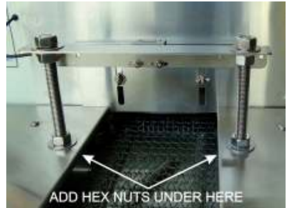
Figure 2-24 Install SENSLAS bracket
