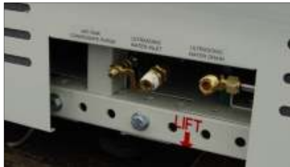
Figure 2-31 UCD Water Connections with Air Purge
