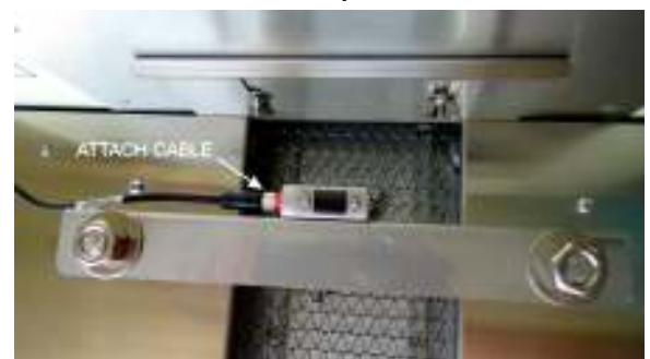
Figure 2-27 Connect SENSLAS cable
