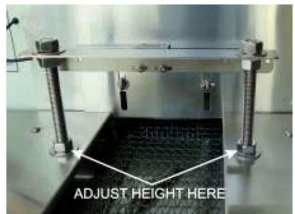
Figure 2-25 Adjust SENSLAS bracket height
