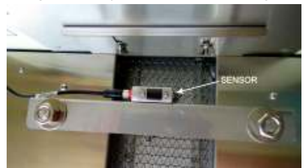
Figure 2-26 Install SENSLAS sensor over center of product lane
