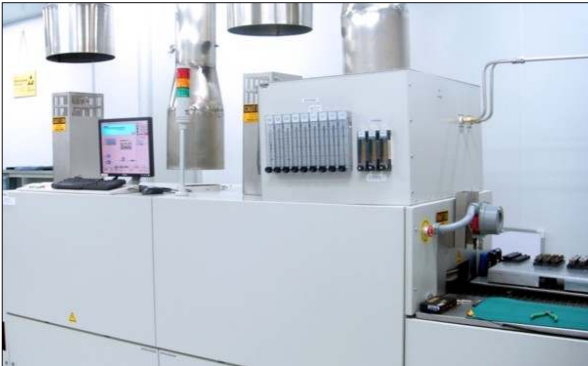
Figure 2-30 Typical Hydrogen Furnace Process Gas Exhaust Connection
