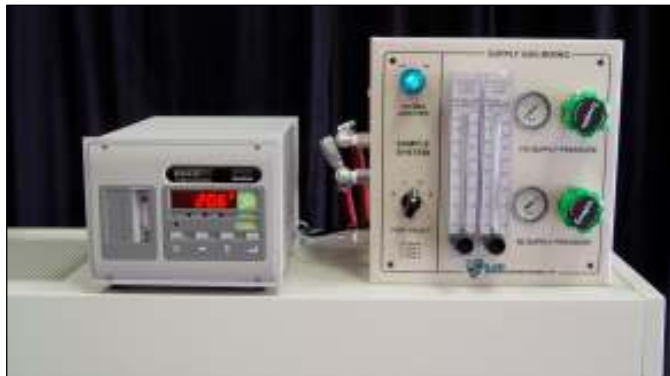
Figure 2-22 Oxygen analyzer on furnace
