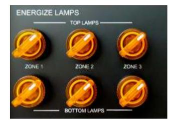
Figure 1-12 Energize Lamps control panel
