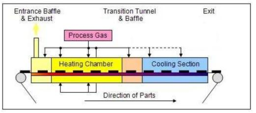
**Figure 1-8 Process Sections**
