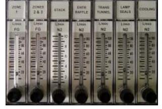
Figure 1-20 Gas Flowmeters - Single Gas
