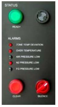
Figure 1-19 Status Panel and Alarm Controls
