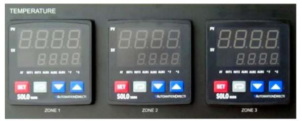
Figure 1-13 Zone Temperature Controllers
