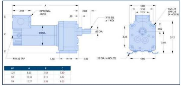
Figure 1-28 Transport Drive DC Motor
