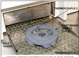
IR FURNACE BRASS FORGING SAMPLE, 720C AT EXIT Figure 9-7 Brass Forging Sample With 2 thermocouples
