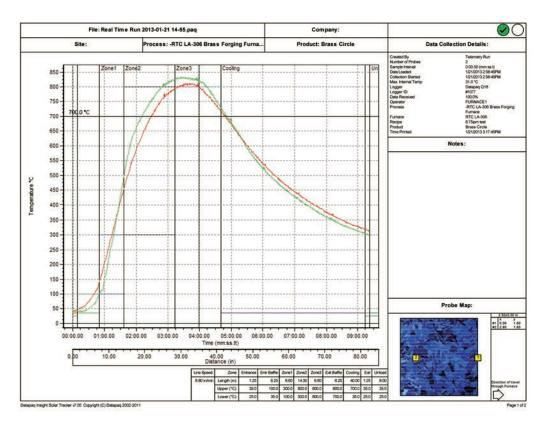
Figure 9-14 880 °C Brass Forging profile
