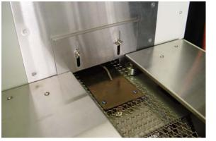
Figure 9-12 Sample plate exiting furnace
