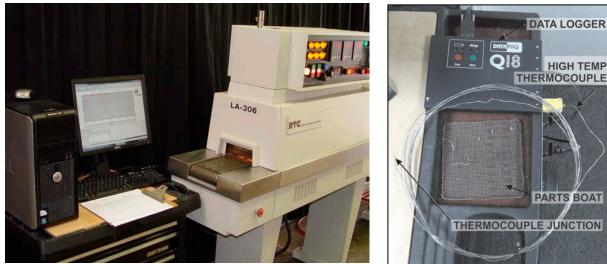
Figure 9-5 Temperature Profiling Apparatus
