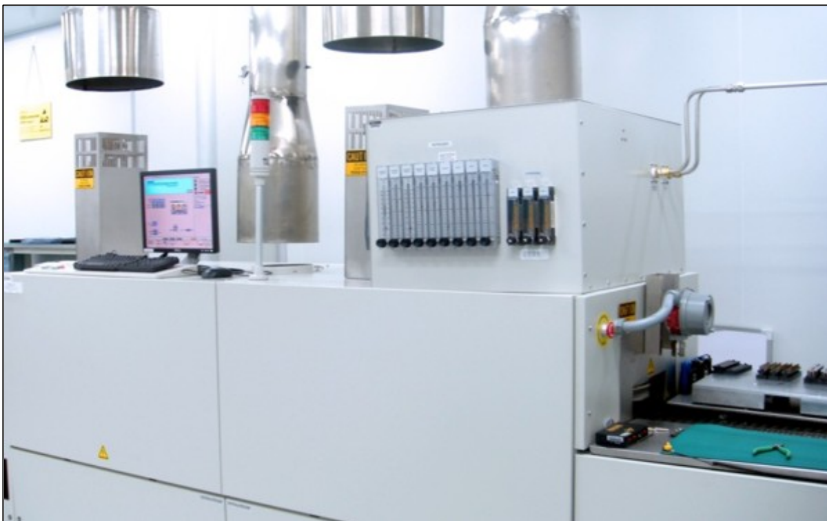
Figure 2-30 Typical Hydrogen Furnace Process Gas Exhaust Connection
