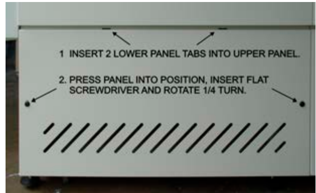
Figure 7-7 Lower Access Panel Installation
