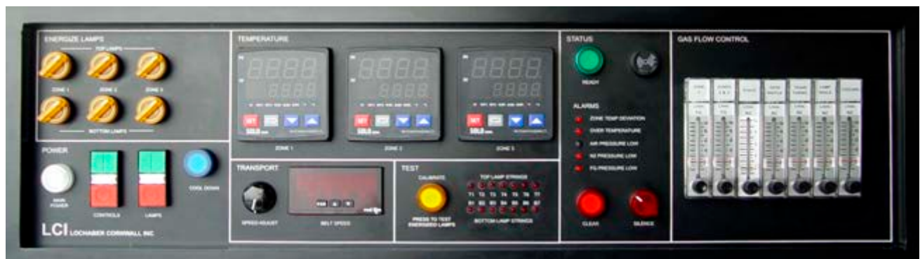
Figure 1-10 LA-306 Control Console
