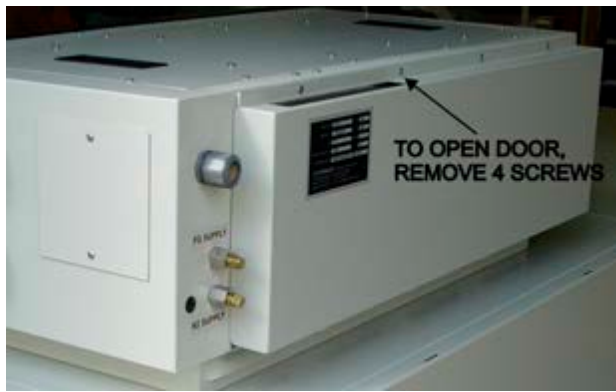
Figure 7-4 Control Enclosure Access Door Closed
