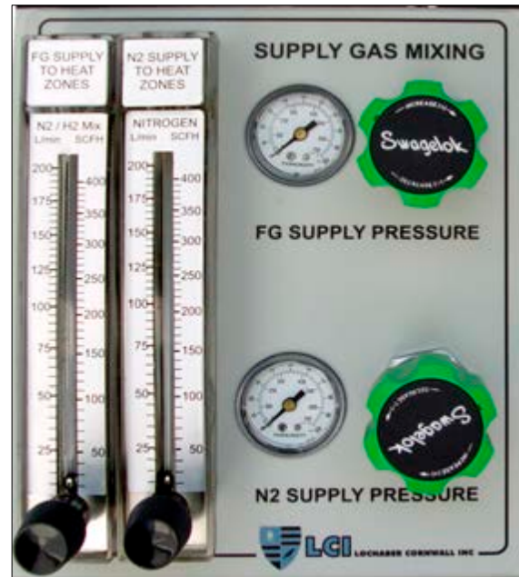
Figure 6-7 Supply Gas Mixing System Control Panel
