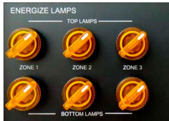
Figure 1-12 Energize Lamps control panel
