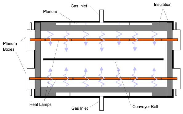
Figure 5-2 Heating Chamber Construction. End view
