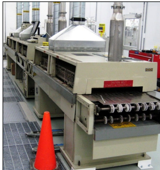
Figure 2-28 Cabinet Exhaust Examples
