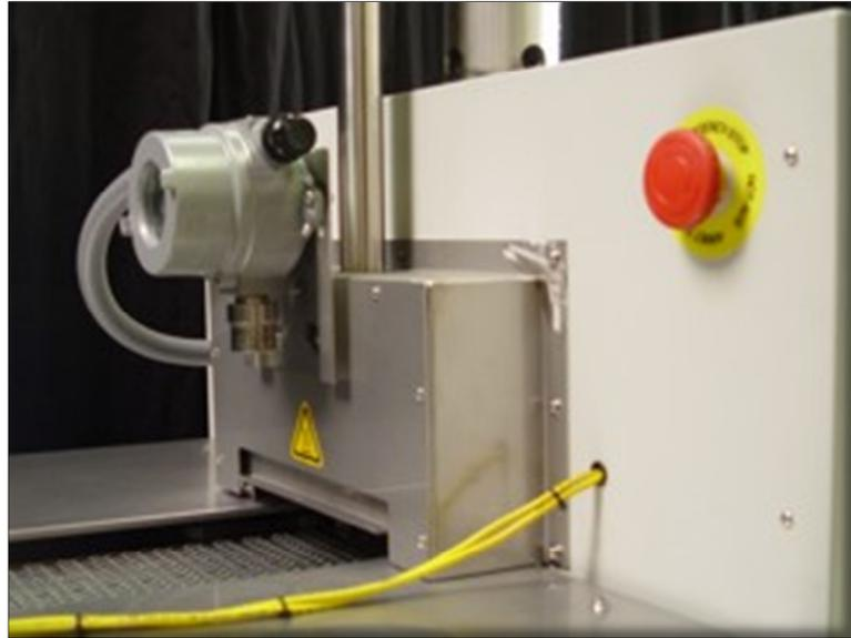
Figure 10.3.8 Gas Collector at Exit
