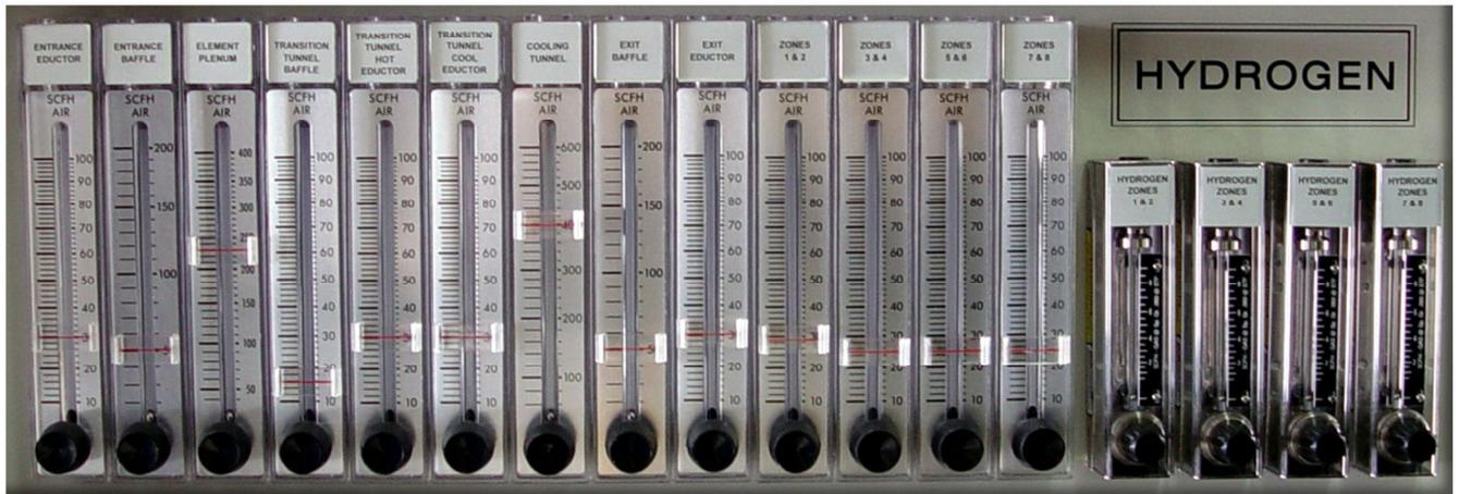
Figure 10.3.2 Nitrogen and Hydrogen Flowmeters
