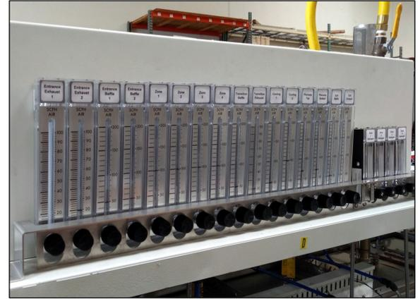
Figure 10.3.1 H2/N2 Mixing System enclosure
