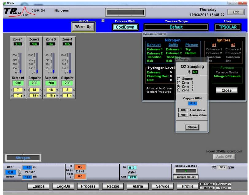
Figure 10.3.6 O<sub>2</sub> Sampling window on Process screen
