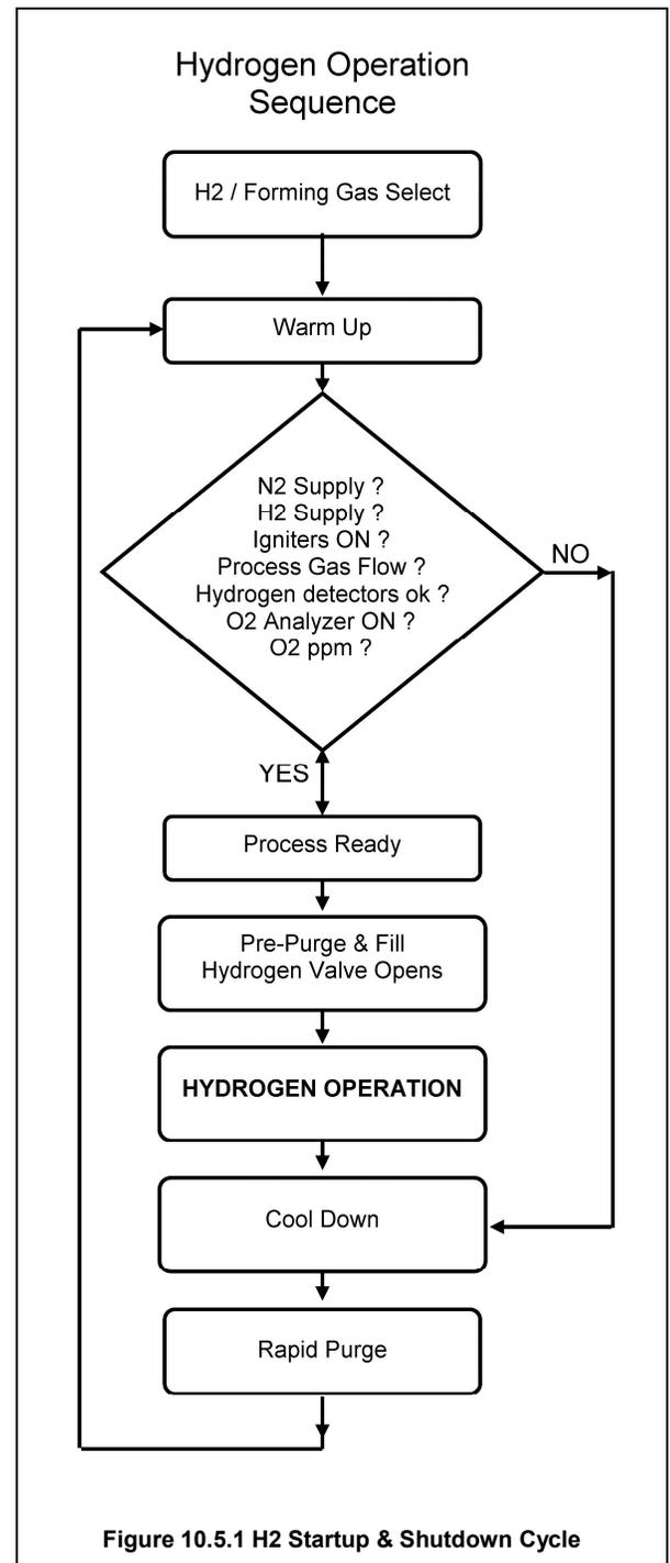
Figure 10.5.1 H2 Startup & Shutdown Cycle
