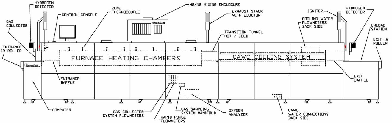
Figure 10.1.1 Typical Hydrogen Furnace
