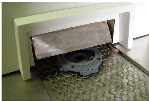
Figure 6-11 Brass forging sample exiting furnace
