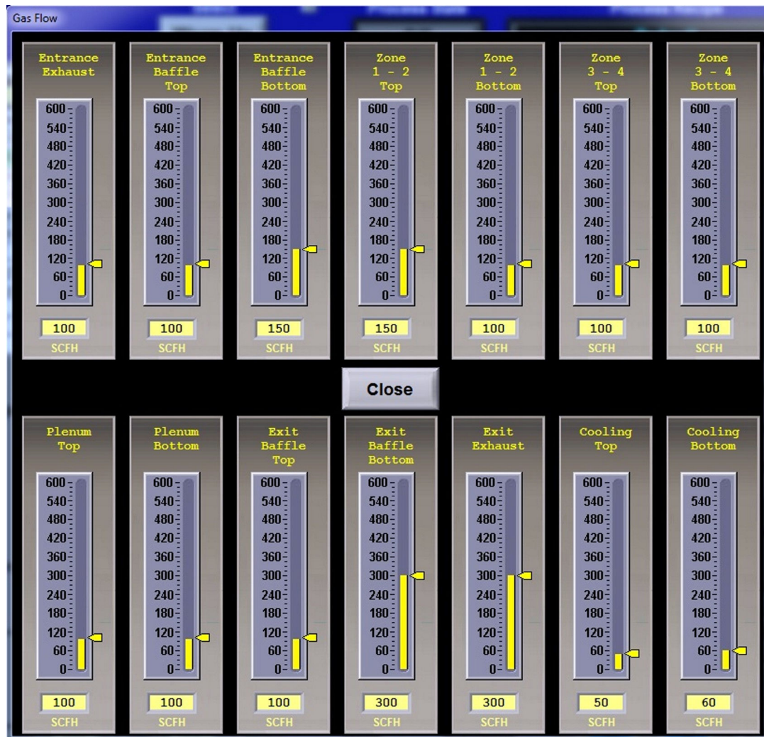
Figure 3-45 Gas Flow Screen
