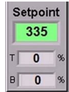
Figure 3-26 Zone Temperature & Power fields
