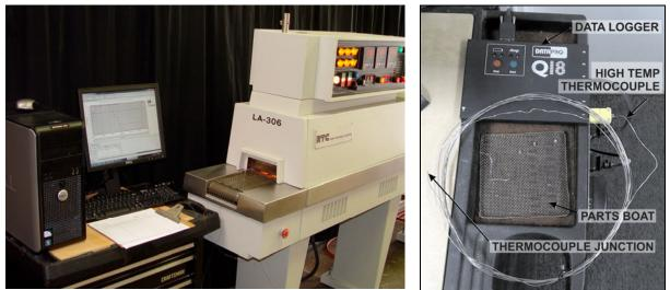
Figure 8-5 Temperature Profiling Apparatus
