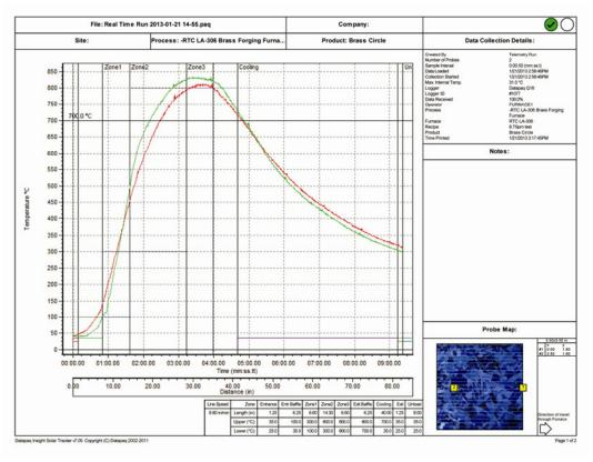
Figure 8-14 880 °C Brass Forging profile
