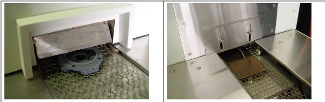
Figure 8-11 Brass forging sample exiting furnace
