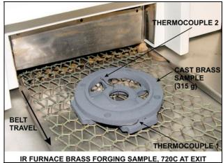
FURNACE BRASS FORGING SAMPLE, 720C AT EXIT Figure 8-7 Brass Forging Sample With 2 thermocouples
