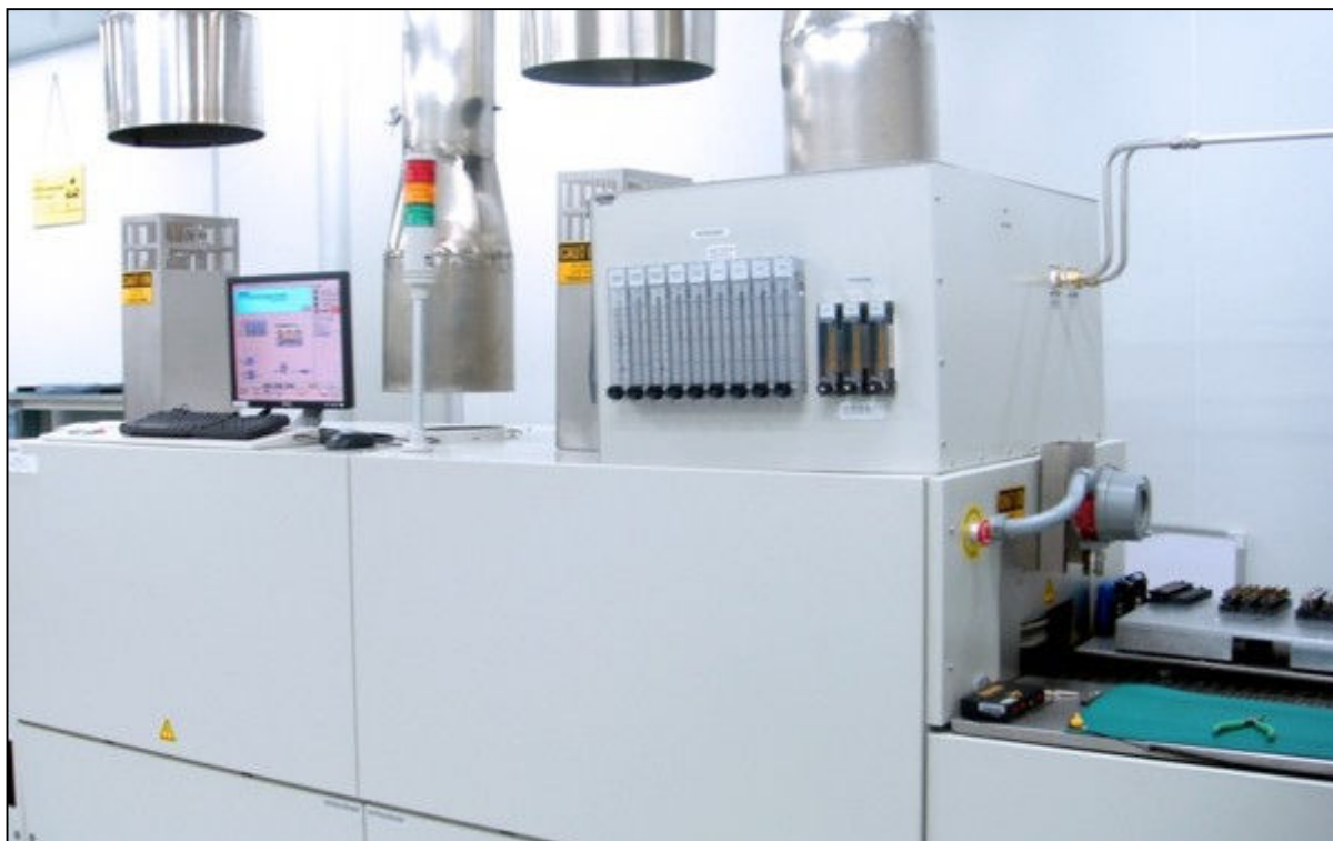
Figure 2-34 Typical Hydrogen Furnace Process Gas Exhaust Connection
