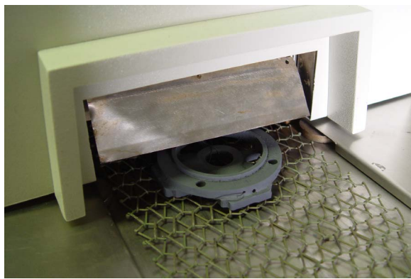
Figure 9-11 Brass forging sample exiting furnace
