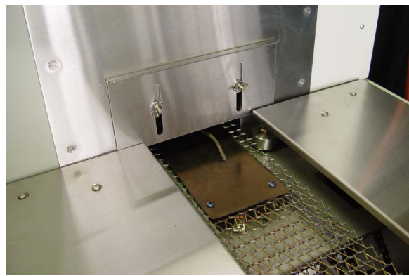
Figure 9-12 Sample plate exiting furnace
