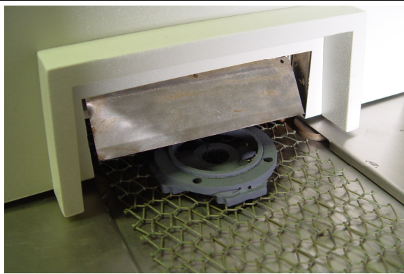
Figure 9-11 Brass forging sample exiting furnace
