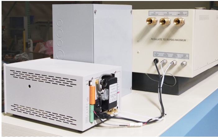
Figure 4-12 Oxygen Analyzer furnace connections
