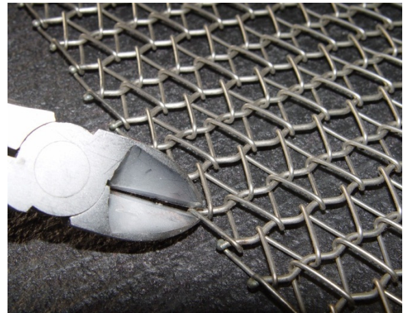
Figure 4-18 Cut wire at ball joint
