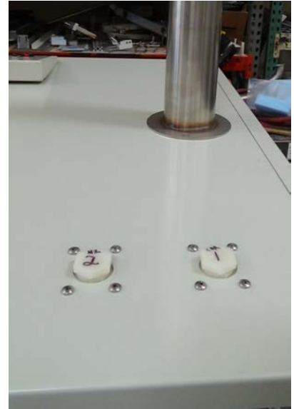
Figure 0-21 Control Enclosure showing Dual Process Gas Connections
