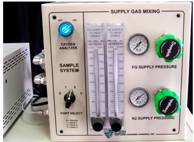
Figure 0-30 Sample System control panel (shown with Supply Gas Mixing System)
