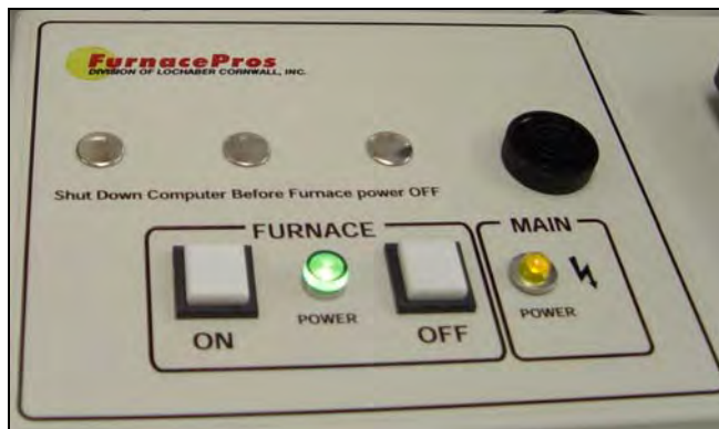
Figure 2.1.1 Control Panel showing Furnace Power ON and OFF and Indicator Lights
