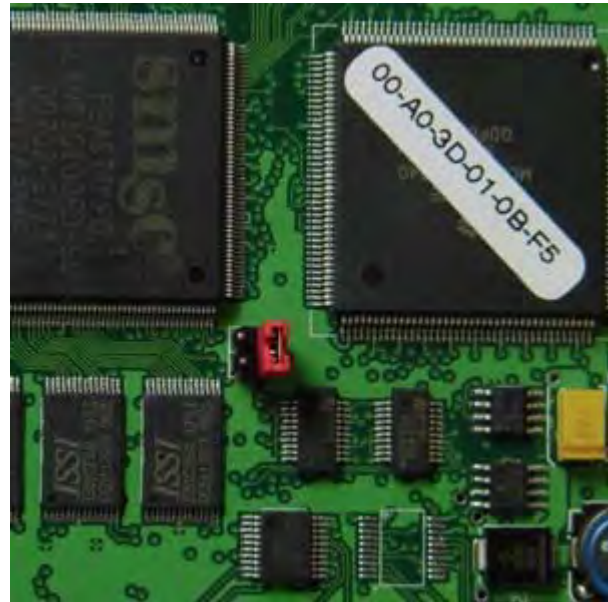
Figure 3.16.6 Move J7 Jumper to Module Reset
