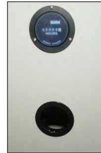
Figure 1.2.4 Power Port and Elapsed Time Meter
