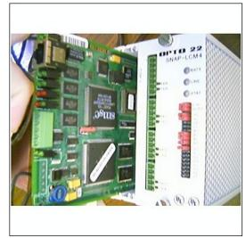
Figure 3.16.4 Ethernet Card Removal
