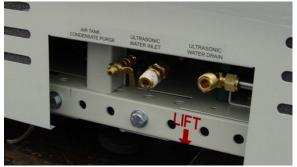
Figure 1.2.13 Water Connections and Air Purge
