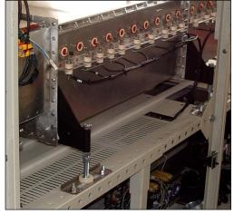
Figure 1.2.2 Leveling Chamber Supports
