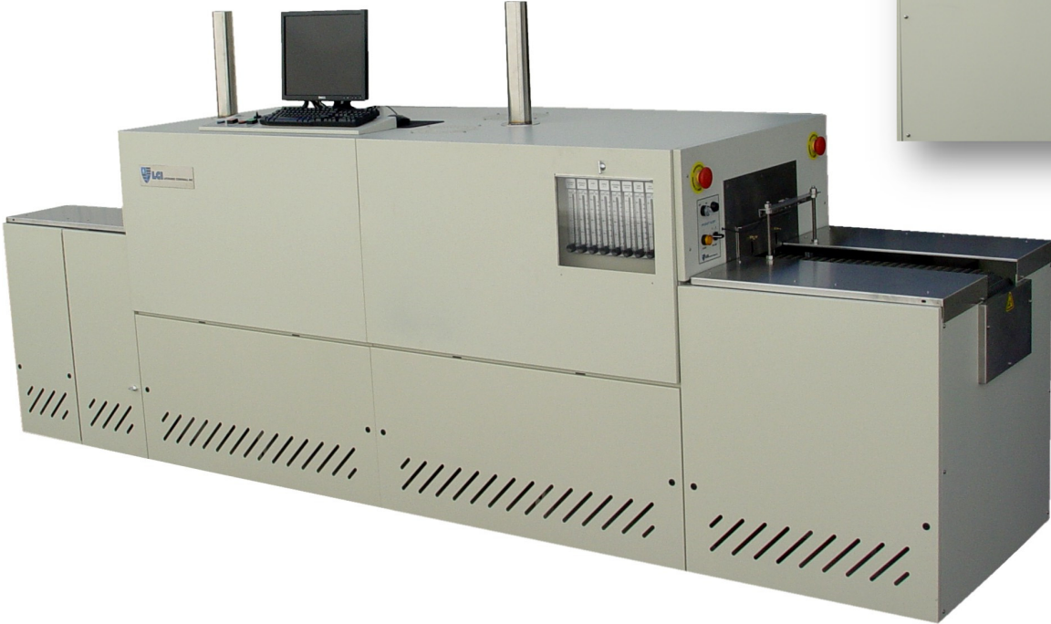
Figure 0-8 Front Exit LA-309 with Exit Extension and SENSAS Product Alert
