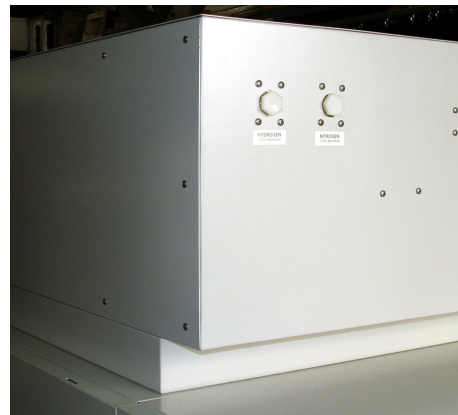
Figure 0-18 Control Enclosure showing Dual Process Gas Connection
