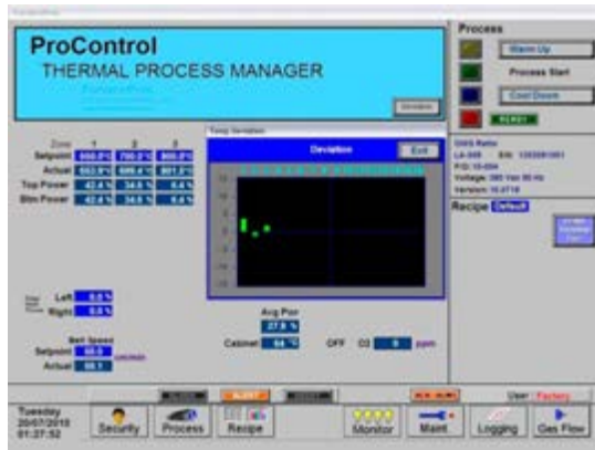
LA-309 Software Process Screen During @ 800 C Profile, Belt Speed: 50 cm/min
